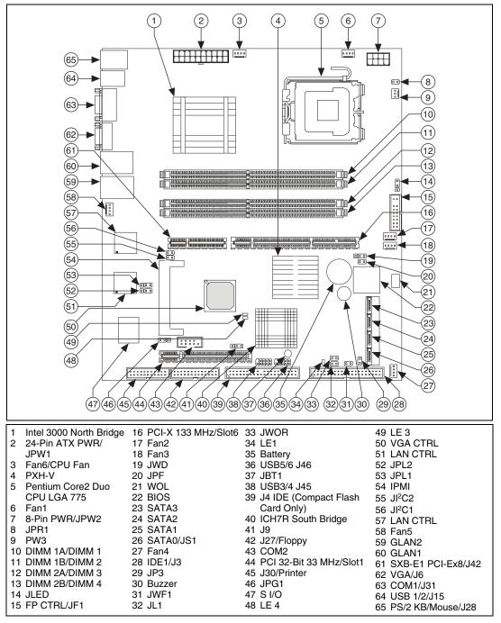
Figure B-1. NI 8352/8353 Mainboard Layout
